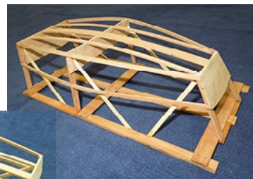
This shows Mills' jig system for making multiple, identical hulls for fleet racing.
