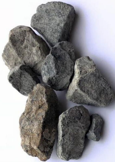
Aggregate 3/4 = 20 MM - 30 MM
