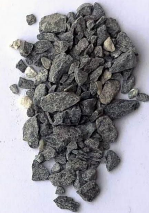
Aggregate 3/16 = 05 MM - 10 MM
