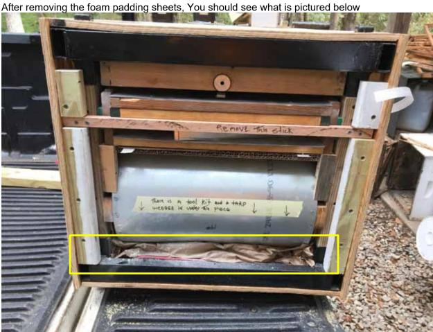
Pull the paper packing material out from under the curved sheet metal near the bottom – yellow square on the picture
