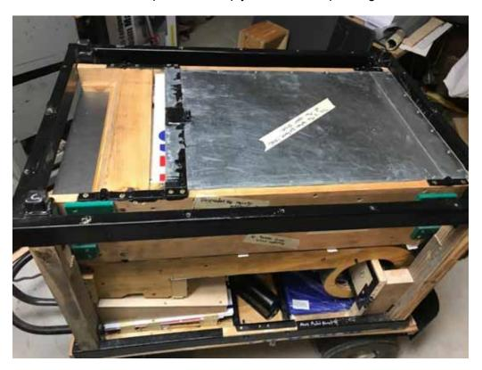
The top shoe (box-frame that holds the screens) is upside down. If the sheet-metal surface that is in view is damaged, it will have to be skillfully flattened or replaced.
