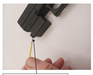
Access holes for laser adjustment. Two on each side. **Example:** To adjust the laser up, loosen the upper right screw (typically about 1/2 turn at a time) and tighten the lower left screw the same amount until the screw is snug. (Do not overtighten the screws.)
