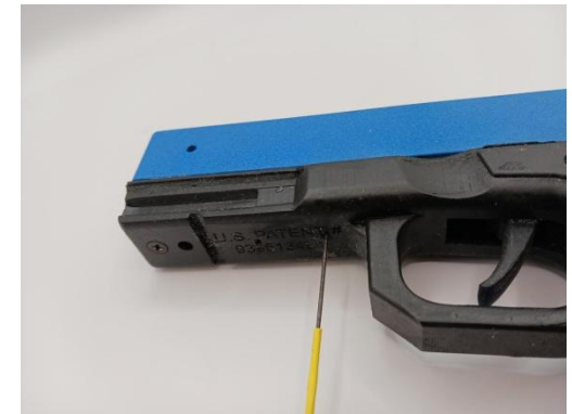
Allen wrench inserted to energize laser
