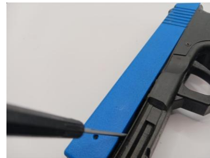
Use thin blade screwdriver to lift slide
