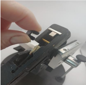
Installing Travel Stop
