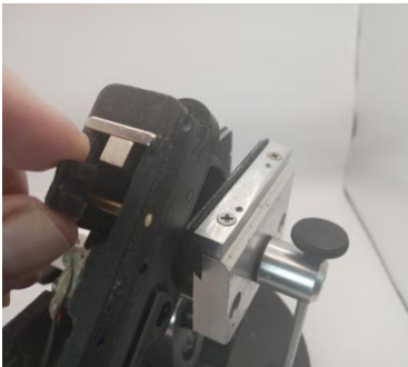
Travel Stop Installed
