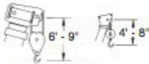
DIMENSIONS ARE FOR LARGEST FACTORY FURNISHED HOOK BLOCK AND HOOK & BALL, WITH ANTI-TWO BLOCK ACTIVATED
