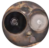
Cylinder head after one P.i. treatment.
