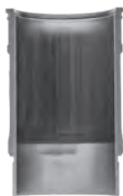
Severely Scuffed Liner
