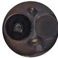
Cylinder head before P.i. treatment.
