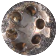
Injector after one P.i. treatment.
