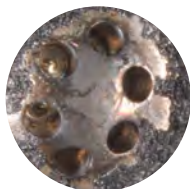
Injector after one P.i. treatment.
