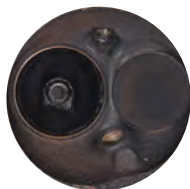
Cylinder head before P.i. treatment.
