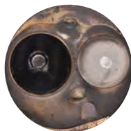
Cylinder head after one P.i. treatment.
