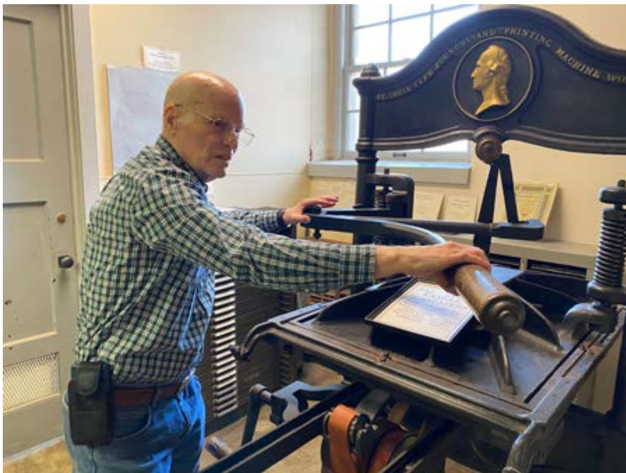
Dennis Duty demonstrates the operation of the restored 1876 Washington Flatbed Newspaper Press. Photographer: Cynthia Rhodes
