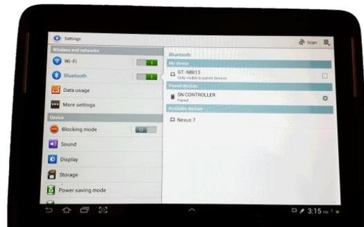
When the tablet is paired with the in-cab controller the system will search for a GPS signal, when this is obtained the system will go into “Smart Nozzle mode. Note: If no GPS is found you will see the error message “No GPS Signal” Check that the GPS receiver is on and receiving a signal.
