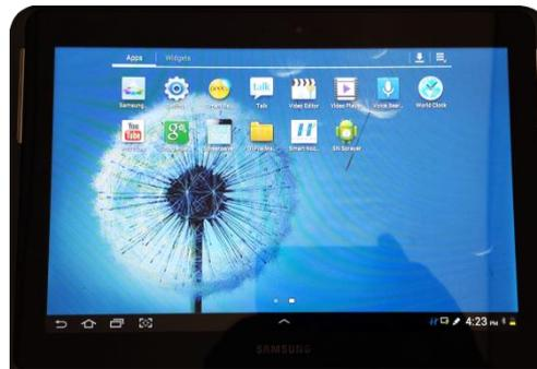
When the software loads you will see the Smart nozzle home screen. The software will immediately search for the in-cab controller via the “Bluetooth” transmitter. This should have been paired to the android tablet during the installation process. If no connection is made you will get the error message “No Bluetooth Connection”.
