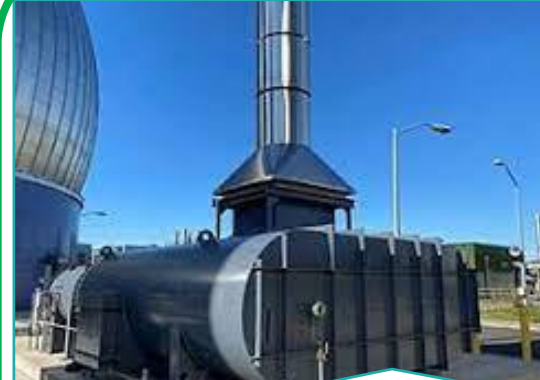
S3 – Regenerative Thermal Oxidizer
