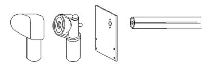
Insert the output shaft of the motor through the large hole of the roller plate. Bolt motor to the plate using (3) 5/16" x 1" bolts with flat washers and lock washers. Bolt the output shaft of the motor through the predrilled hole in the roller tube using a 5/16" x 2 1/2" grade 5 hex bolt and nylock nut.
