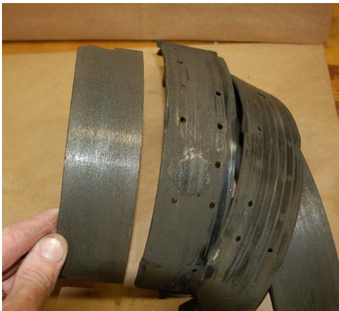
The lining face looks normal, no cracks, etc
