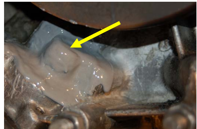
JB Weld applied over shaft bore.
