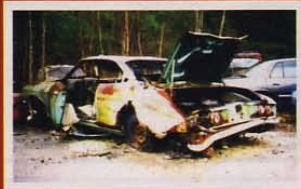
The body-colored taillight cove tells us it's not a '65 to '66 Corsa. The Corsa, Corvair's muscle model, had an argent silver cove and a standard 140hp four-carb engine. The 180hp turbo engine was optional. Another non-Corsa giveaway is the standard three-pod instrument cluster. Corsas featured a six-gauge cluster.
