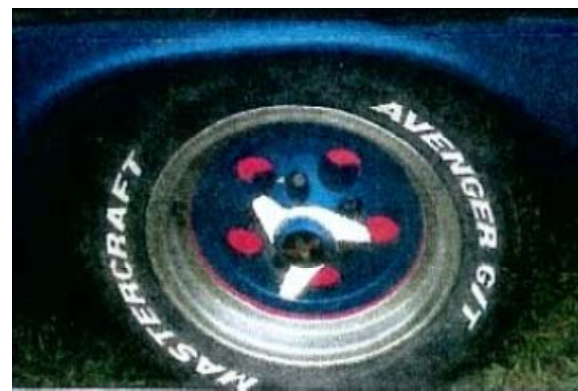
Reflective disks mounted behind the wheel for added visibility and to hide the drum. Red stripe around the blue wheel center also adds to night visibility. Spinner is reflective also.
