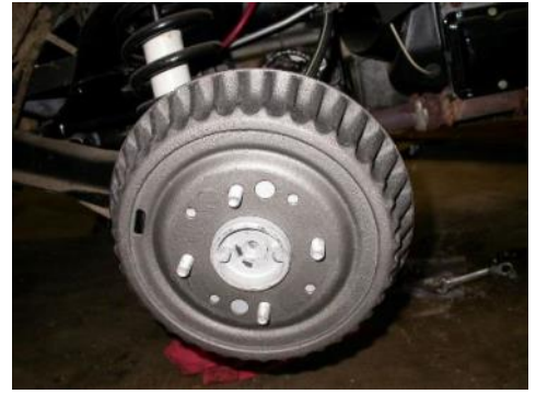
Axels in, drums painted and installed
