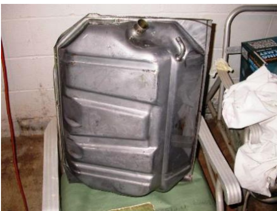
Fuel tank, cleaned, acid etched and painted with POR15 clear. Next...coat the inside with POR's gas tank sealer.
