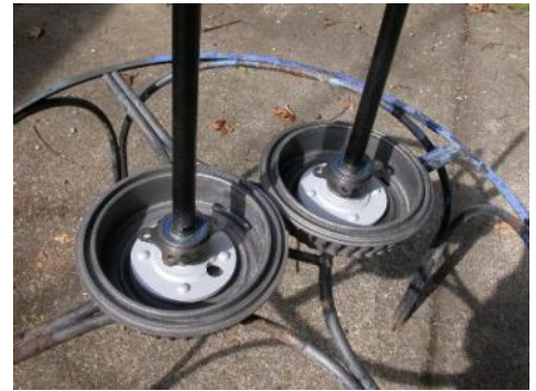
Axels cleaned, painted and new wheel bearings installed
