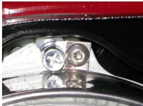
Details of headlight fastening
