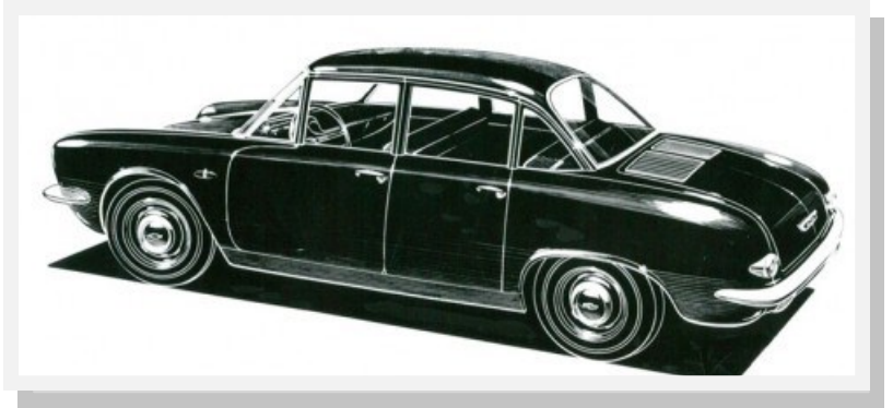
Artist's conception of the small Chevrolet based on trade reports. This drawing shows air intake for flat six-cylinder engine behind rear window. Model is expected to have more room than an average imported economy car. December 18, 1958
