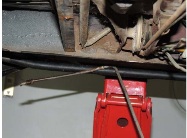
View of the old brake line after removal from the tunnel. You can see the pulley for the clutch cable.
