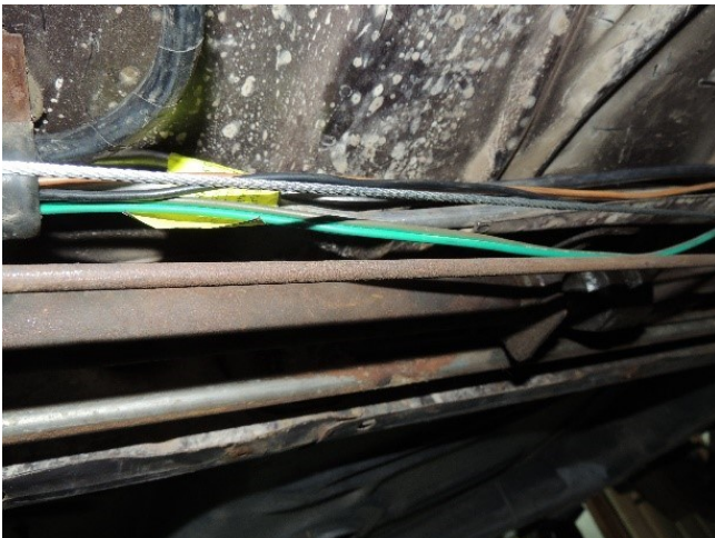
This is the picture that saved me. It shows the brake line in relation to the emergency brake cable, and how they properly cross in the tunnel to avoid rubbing together.
