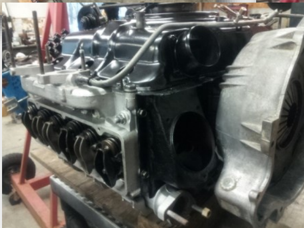
New fan bearing. Jugs have been polished and cross hatched.
