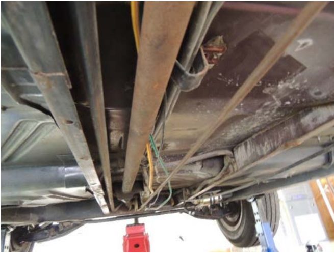
View of tunnel looking to the front of the car. Note the shift tube and clutch rod.
