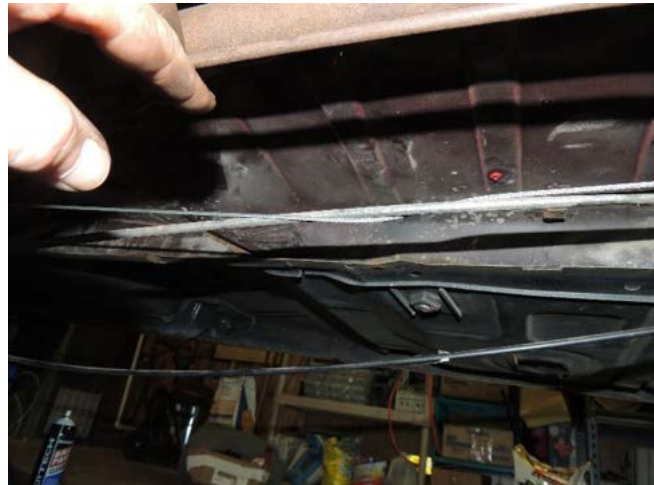
First attempt to install the line in the tunnel. Got the brake line twisted around the emergency brake cable. Remove and repeat (this is where the nerve medicine comes in handy!)
