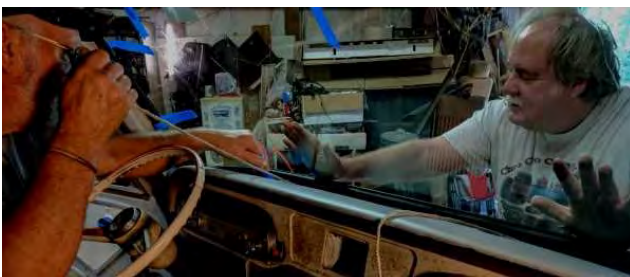
Pressure is applied from outside while pulling the rope from the inside which effectively forces the rubber over the metal lip.
