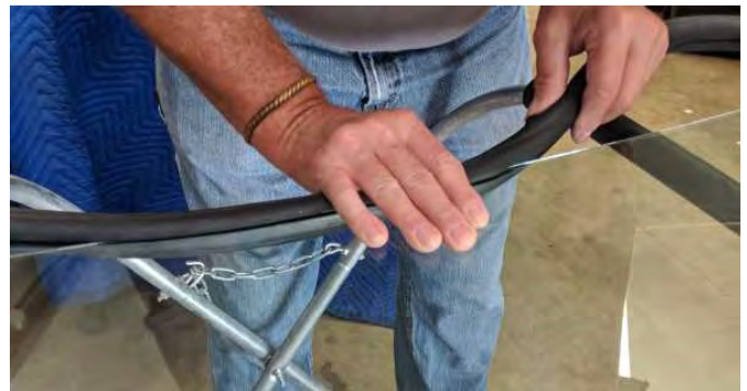
A trial fit of the window moulding to ensure it is in the proper orientation..
