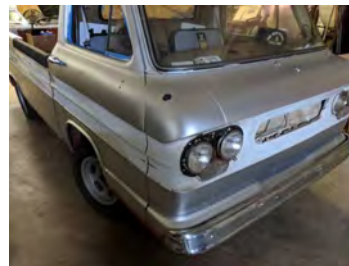
The gray base coat over the faded and prepped original red. Three coats with 24 hours cure between each.
