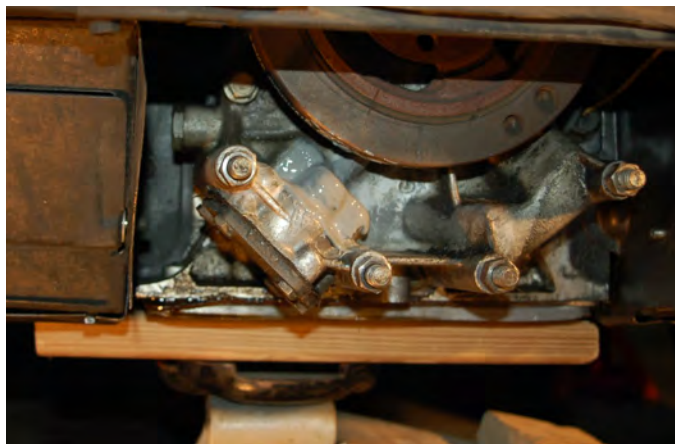
Engine support for lowering and access.
