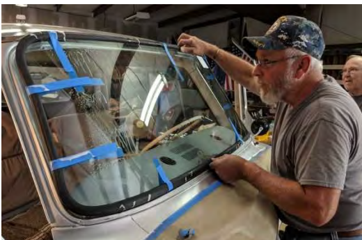
Liberal amounts of ammonia free glass cleaner is applied on ALL surfaces before placing the windshield...
