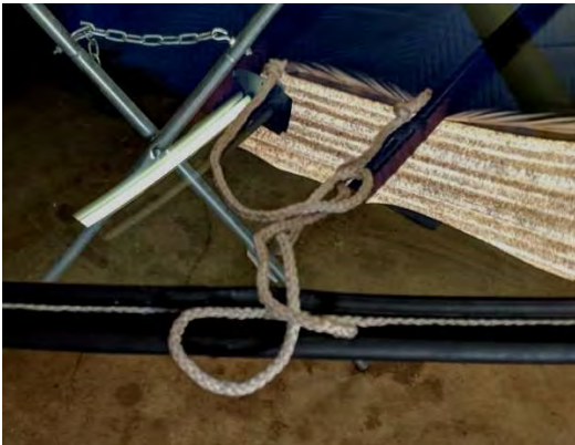
Rope placed inside window molding to facilitate fitment on the inside of the cab.
