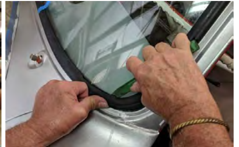
As I stated in the text, the corners just do not fit well. Stan manipulated and coaxed the rubber with his 'bone tool' until it got kinda close. It may improve as the rubber stretches out a bit. We will see.
