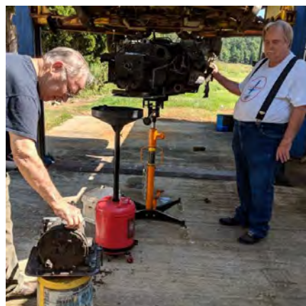
Jack did a fine job fabbing up his homemade cradle for the power Pack removal. It just needed a little friendly persuasion from a nearby hammer.
