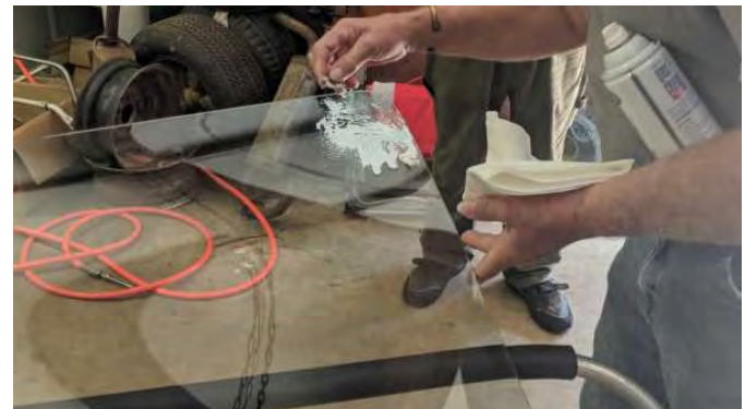
Ammonia free glass cleaner must be used (for lubrication) when removing stickers with a razor blade..
