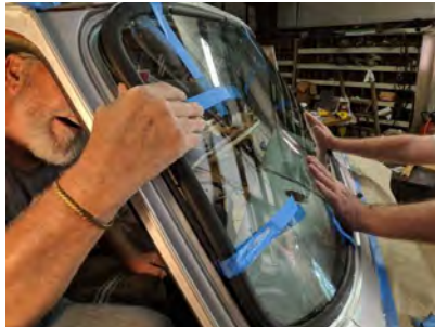
As I stated in the text, the corners just do not fit well. Stan manipulated and coaxed the rubber with his 'bone tool' until it got kinda close. It may improve as the rubber stretches out a bit. We will see.
