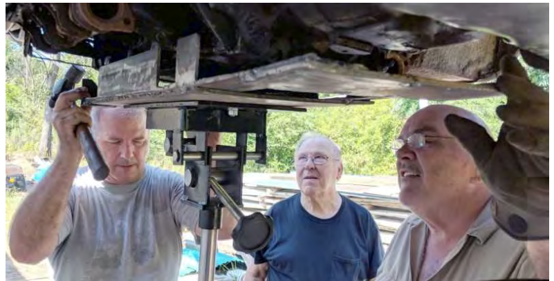
Jack did a fine job fabbing up his homemade cradle for the power Pack removal. It just needed a little friendly persuasion from a nearby hammer.
