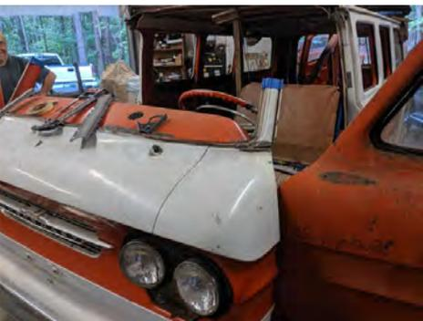
Here the drivers side pillar has been cut 'long' to facilitate a 'trim as necessary' approach.
