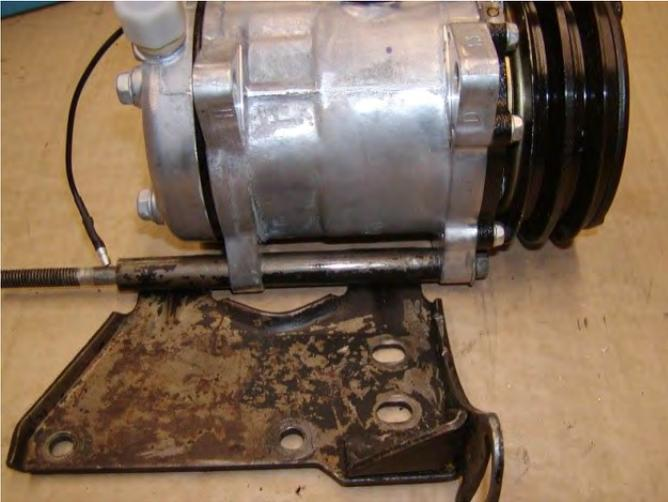
Taking the original bracket we cut out a section of pipe to accommodate the ear on the Sanden compressor
