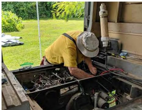
Note the PVC pipe IV fuel system hanging next to Russ. Ideal temporary fuel bypass solution.
