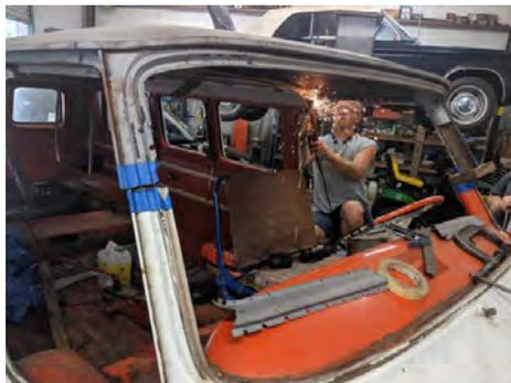
Mark is making angle cuts for fitment of the roof at the 'B' pillars
