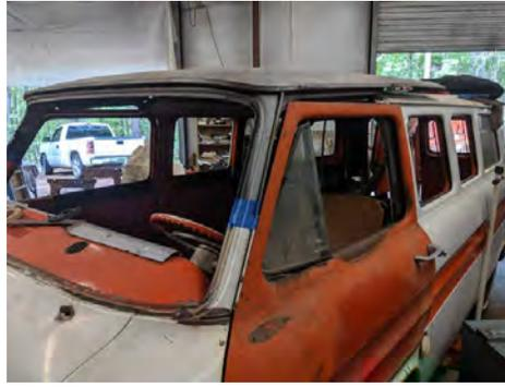
Mark says; "Measure fourteen times and cut just once!" The donor roof was lifted into place for trial fit many times!
