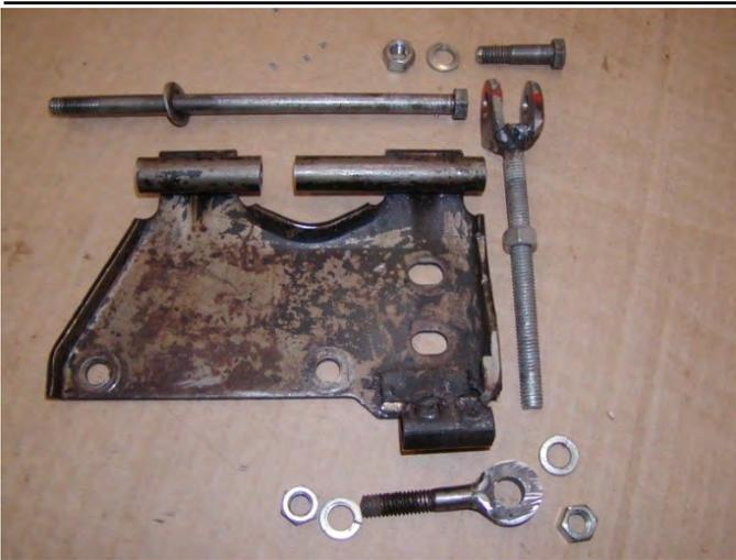
The third and final modification is to weld a short piece of pipe or tube to the bracket to accommodate the bolt with a spacer welded on it to adjust belt tension
