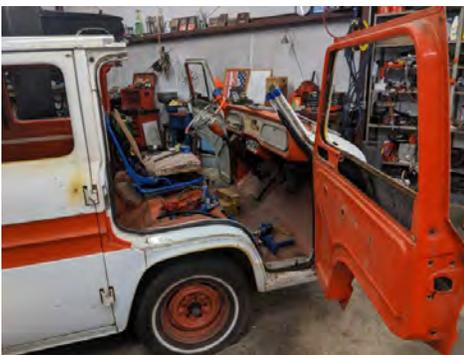
The 'A' pillars have been cut for preliminary measurements compared to the donor roof's pillars.
