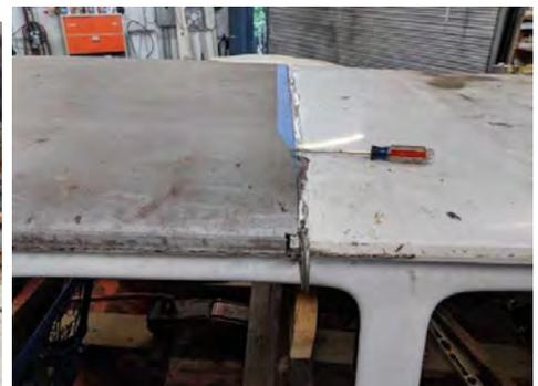
The roof sheet metal is very thick but will take a bead nicely.
