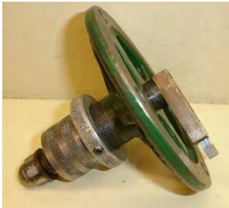
The large knurled ring has depth setting numbers on the top. VAIRMECH provides this description; "This one has no cylinder centering so you
