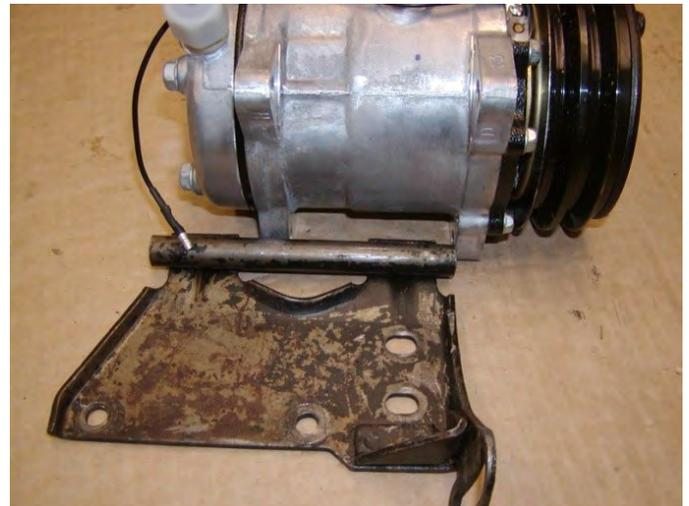
Next we cut off the ear with the slot in it that adjusts the compressor belt tension
