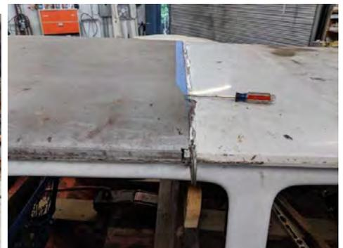
The roof sheet metal is very thick but will take a bead nicely.
