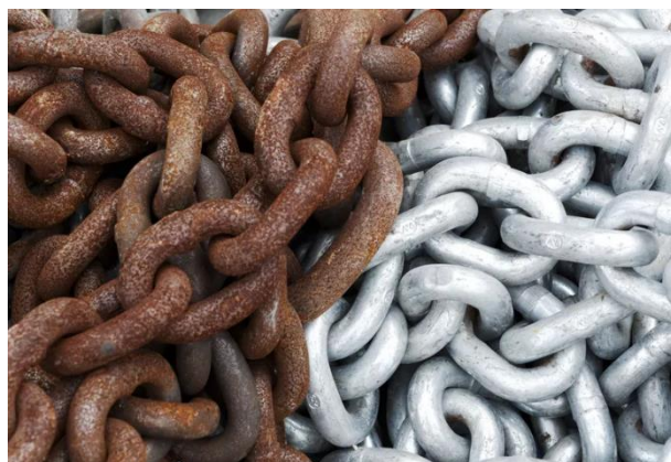
Figure 3. Example of a chemical change as metal chains rust over time. The chains on the left have rusted. The chains on the right have not because they have a special coating that prevents them from rusting. Source: photostock-israel/getty images
