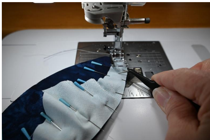
Sew a \frac{1}{4} " seam following the shape of your curve. Use your tweezers to adjust and hold your top piece.
