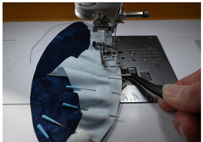
Sew a \frac{1}{4} " seam following the shape of your curve. Use your tweezers to adjust and hold your top piece.
