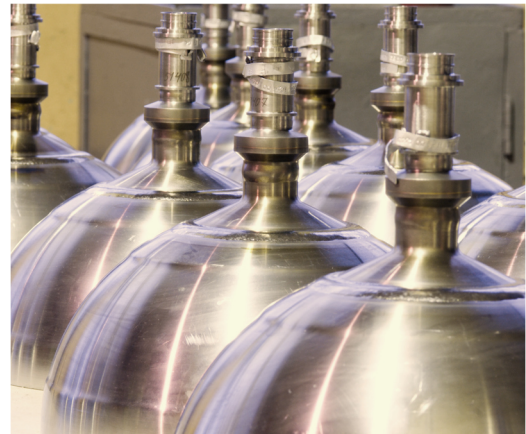
Stainless Steel Tanks for 300 bar MEOP
