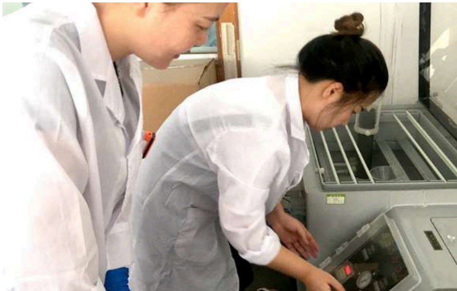
Hardware Salt Spray Corrosion Test
