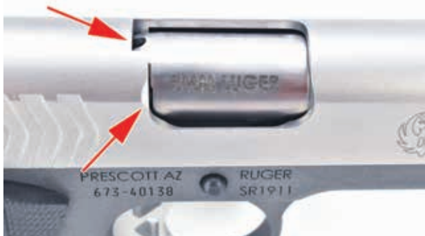
Above: The ejection port has been properly lowered and slightly relieved at the rear (bottom arrow). The barrel hood is notched at the rear (top arrow), allowing a small viewport to check for a loaded chamber.
