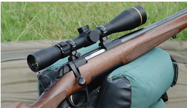
Browning goes above and beyond with scope rings that attach with eight screws instead of the standard four. The glass will stay put.
