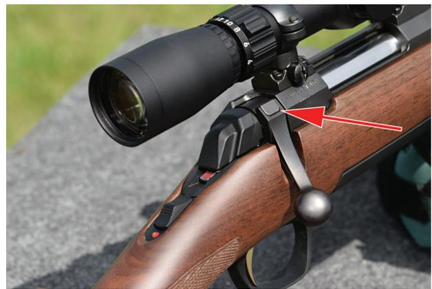
The button on the bolt handle allows the shooter to work the bolt while the trigger is locked.
