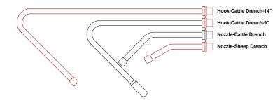
All delivery nozzles have a specific base that is machined or molded to critical dimensions. The base of the nozzle interfaces intimately with the interior of the barrel valve assembly contour. The valve assembly is retained inside the nozzle's base which forces the ball valve against the barrel outlet channel.
