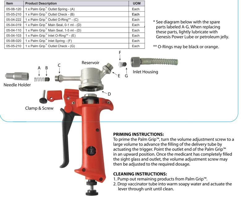
For more thorough cleaning, remove the Clamp & Screw. Hold the Palm Grip<sup>™</sup> in one hand twisting the Reservoir counterclockwise to remove from the body. Clean with hot water. Unscrew the Inlet Housing and Needle Holder to expose the check balls and springs. O-rings and check balls may be lubricated with petroleum jelly to prolong life.
