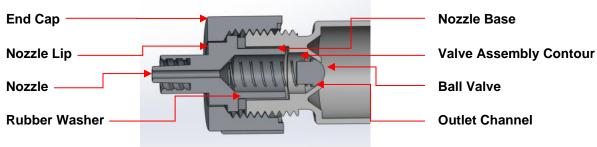
The nozzle's lip expands from its base flaring out to match with the barrel's valve assembly contour and uses a rubber washer to create a tight seal between the nozzle and barrel. The end cap surrounds the nozzle's lip and threads directly onto the outside diameter of the barrel's valve assembly contour.
