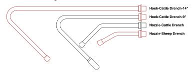
All delivery nozzles have a specific base that is machined or molded to critical dimensions. The base of the nozzle interfaces intimately with the interior of the barrel valve assembly contour. The valve assembly is retained inside the nozzle's base which forces the ball valve against the barrel outlet channel.
