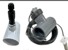
Paddle Sensor, PVC Tee Assembly Kit w/ Stenner Injection Port Flow Range 77428 - 1.5" 900 - 9,000 gal / hr 77431 - 2" 1,800 - 18,000 gal / hr 77434 - 3" 3,600 - 36,000 gal / hr
