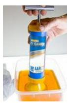
8. Repeat 4 to 5 times to flush the cleaning fluid through the rollers and bearing cage. Inspect bearing and repeat if necessary.
