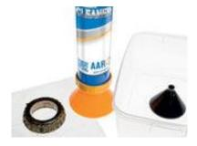
4. Place the black cone plug – point upwards – in the container. Place the bearing – large diameter upward – on the cone as shown.
