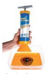
7. Place the yellow cone over the bearing and slowly draw cleaning fluid through the bearing by aggressively moving the piston handle up and down.
