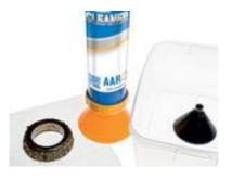
4. Place the black cone plug – point upwards – in the container. Place the bearing – large diameter upward – on the cone as shown.
