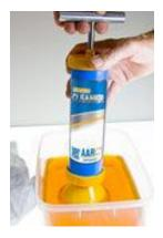
8. Repeat 4 to 5 times to flush the cleaning fluid through the rollers and bearing cage. Inspect bearing and repeat if necessary.
