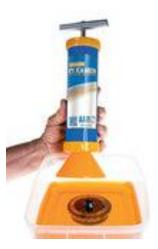
7. Place the yellow cone over the bearing and slowly draw cleaning fluid through the bearing by aggressively moving the piston handle up and down.
