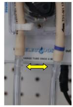
Using the tube connectors provided, connect the pump tube as shown.
