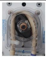
Replace the pump cover and the 3 screws. The tube can be primed using the on-screen controls once the cover is re-fitted.
