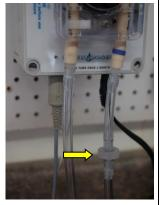
Finish connecting the delivery tube as shown.
