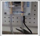
To fit the check valve, cut a piece off the clear tubing long enough to reach from the OUTSIDE of the pump tube to the valve.
