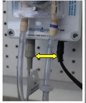
Connect the flow sensor plug along with the power supply.
