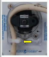
Place the tube restraint in the left hand (IN) side of the pump head as shown. Select "Yes" from the "Load Tube?" screen.
