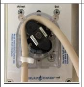
With the rollers pulsing, guide the pump tube around the rollers until it lays in the output notch on the right side of the pump housing.
