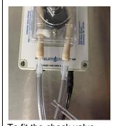
To fit the check valve, cut a piece off the clear tubing long enough to reach from the OUTSIDE of the pump tube to the valve.
