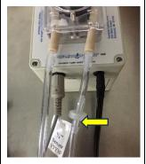
Finish connecting the delivery tube as shown.
