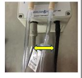
Connect the flow sensor plug along with the power supply.
