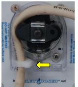
Place the tube restraint in the left hand (IN) side of the pump head as shown. Select "Yes" from the "Load Tube?" screen.
