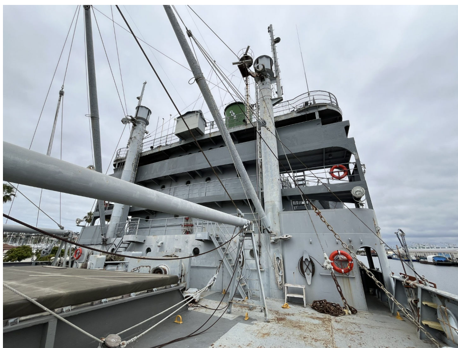
Bridge Front—The Hatch to the No. 3 Cargo hold and more derricks and booms
