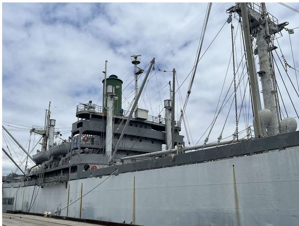
Starboard Side – The main deck house and funnel are situated amidships. Note the dual 20mm anti-aircraft guns above the bridge.
