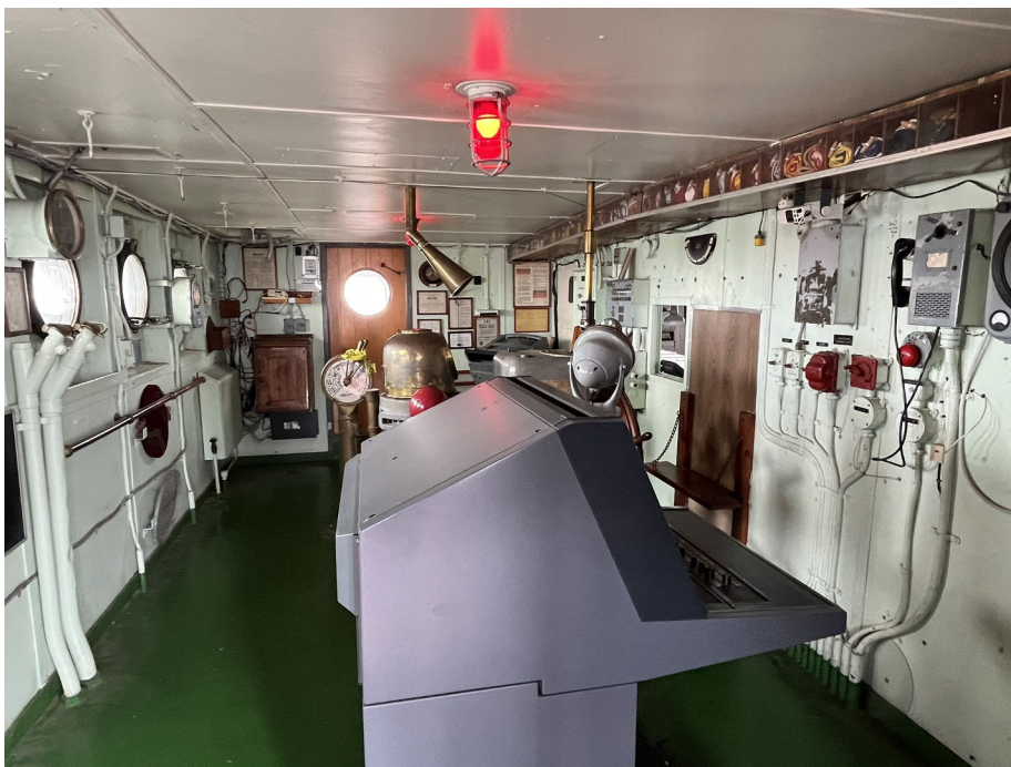
Bridge—Binnacle, helm, radar and engine telergraphs on the bridge
