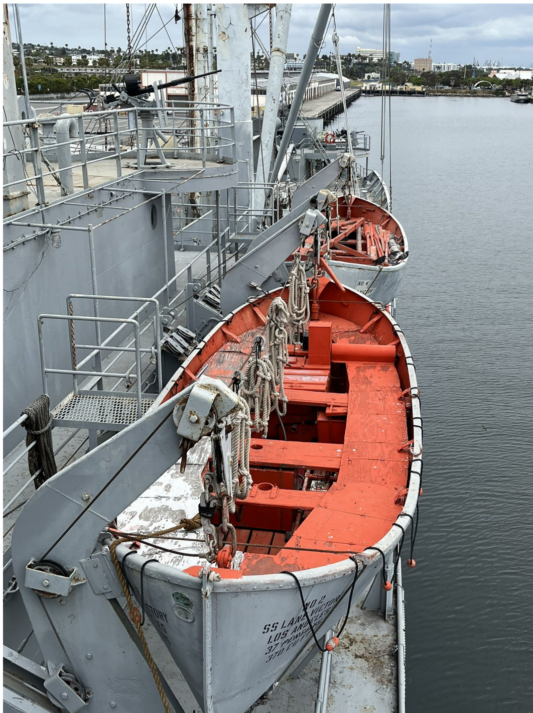
Lifeboats—Four lifeboats on gravity davits were the standard
