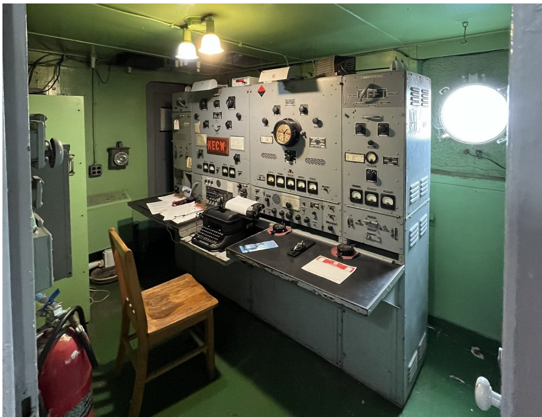
Radio Room—Radio silence was observed twice an hour at 15 and 45 past, to listen for distress signals
