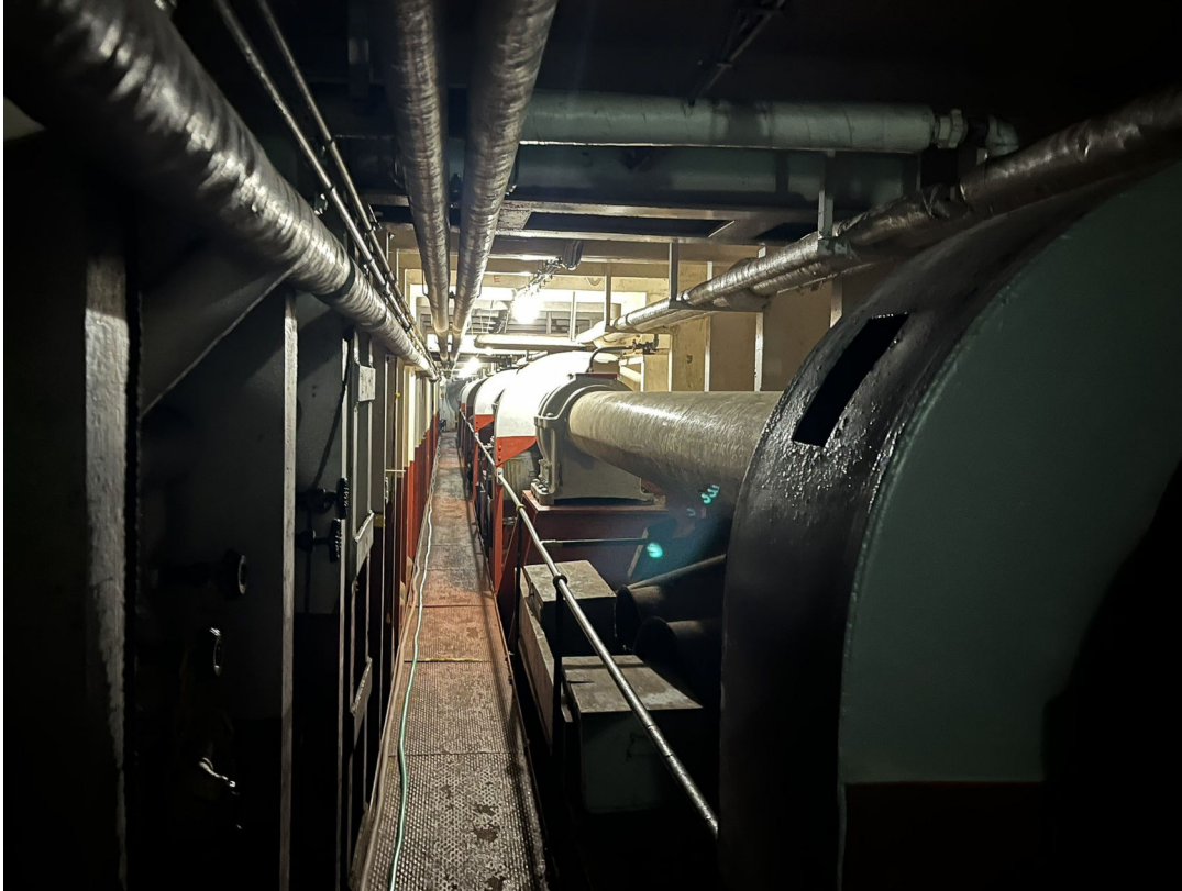
Propeller Shaft—Or “Shaft Alley” leads from the engine room amidship to the propeller at the stern and passes under cargo holds 4 and 5
