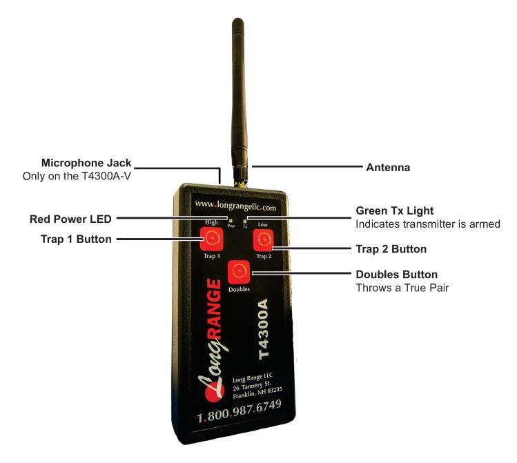
Press any button to power on the transmitter. Be aware the this first button press, even though the device is off, will fire the corresponding trap or traps. The **Red Power LED** will illuminate to let you know that the device is on and ready to launch the second target.
