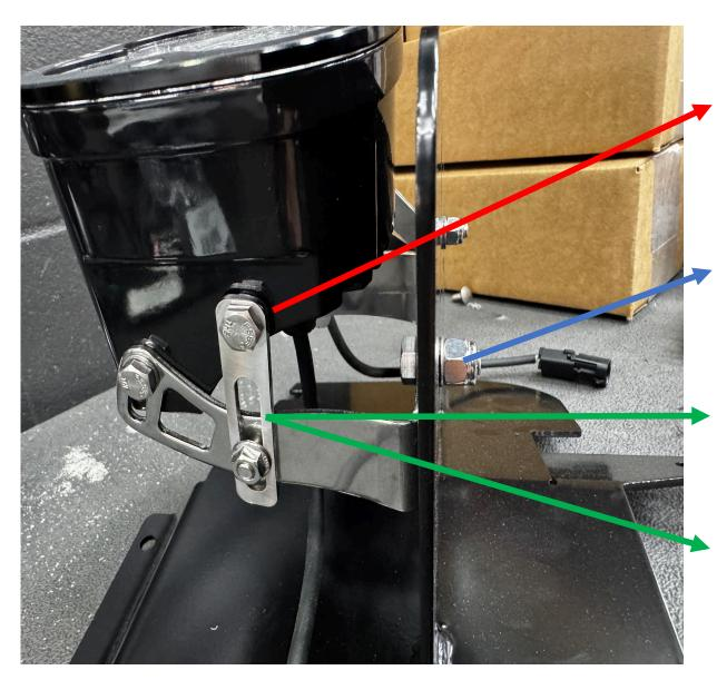
INSTALL SMALL WASHER BETWEEEN LIGHT AND USE HARDWARE THAT CAME WITH LIGHT TO ATTACH THE "UPRIGHT BRIDGE"
