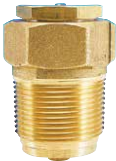
LF 25C Liquid withdrawal Excess Flow Valve. Performance: excess flow closes 4.5÷5.5 m 3 /h (water); residual flow ≤ 0.050 m 3 /h (water) with ΔP +1 bar
