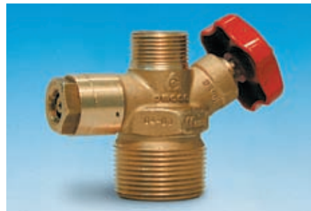
3 Mod. GS-90 - 67.0796 (undergr.) Multiservice Valve (See page Ae1) Multiservice Valve with built-in safety relief valve. When valve VRN-SL and service valve GS-90 are installed on underground tanks a traditional pressure relief valve could be needless. That is because underground tanks are not subject to fire engulfment. Our service valve GS-90 is equipped with a pressure relief device, which is enabled to discharge liquid at 14 bar (setting point).
