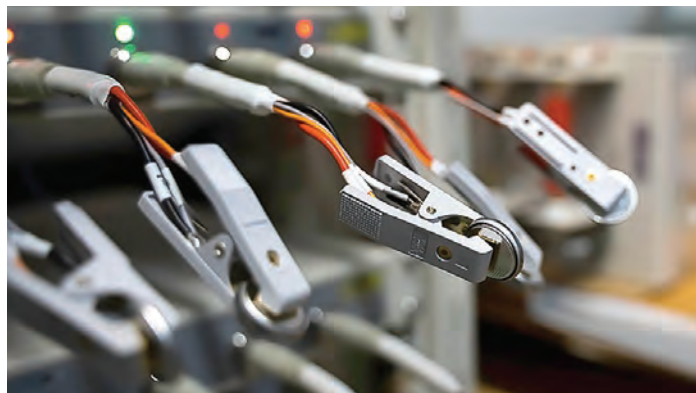
Quasi-solid-state lithium-tellurium battery cells being tested at UBC Okanagan’s Advanced Materials for Energy Storage Lab.
