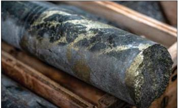
Core from a highly mineralized intercept encountered during 2021 drilling of the East Ridge discovery on the Red Chris gold-copper project in BC.
