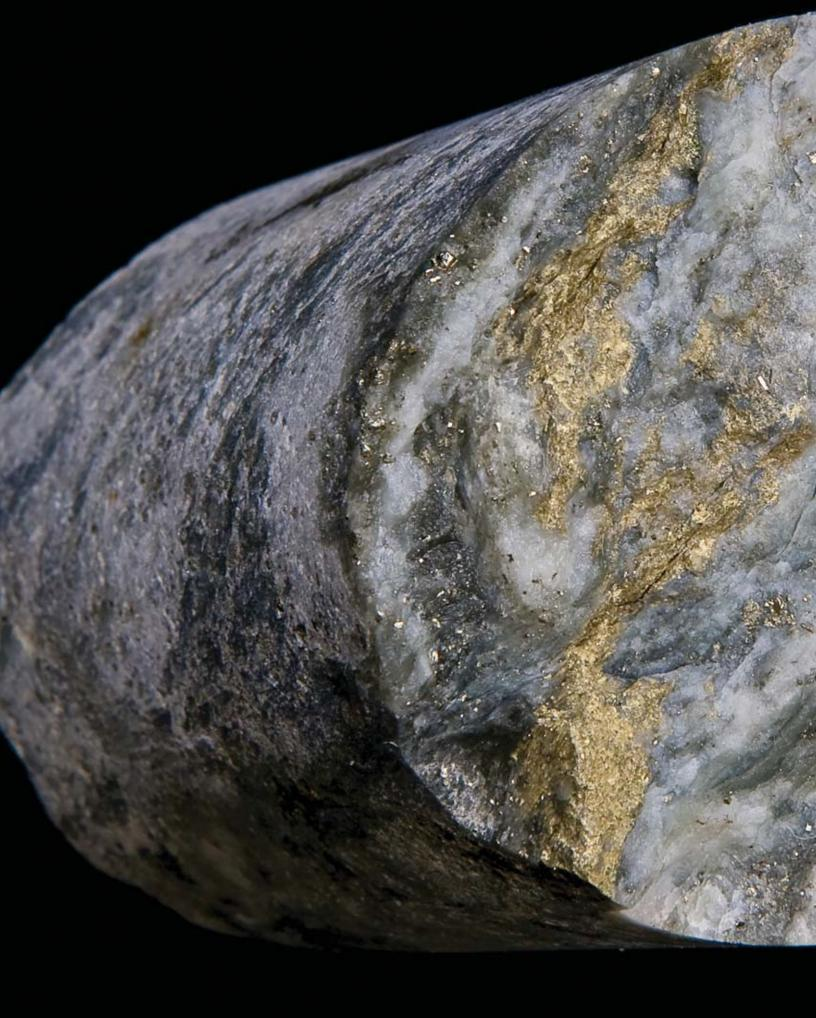
Bonanza-grade gold in core from a hole drilled at Newcrest Mining's Brucejack Mine in Northern British Columbia. PRETIUM RESOURCES INC.
