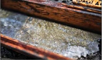
Core from drilling into the gold-rich VMS mineralization at Eskay Creek.
