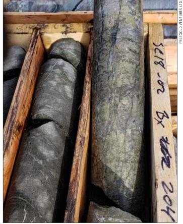
Core from a 2018 hole drilled at Shorty Creek that cut 442.4 meters averaging 0.22% copper, 0.13 g/t gold, 4.03 g/t silver, and 0.02% tungsten.
