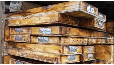
Boxes of core from drilling at Giga Metals' Turnagain nickel-cobalt project.
