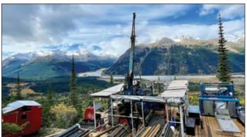
Teck completed 4,688 meters of metallurgical drilling during the 2022 season at the Schaft Creek porphyry copper project in Northern British Columbia.
