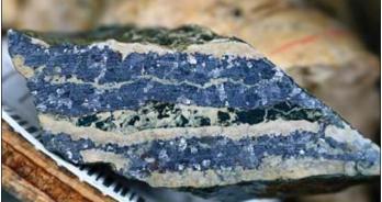
This sample is from a 1.1-meter intercept from drilling at Alianza Minerals' Haldane project that averaged 3,010 g/t silver, 6.4% zinc, and 5.4% lead.
