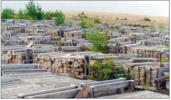
Acres of drill core from past operations at Pine Point. Approximately two to three football field lengths across and eight to 10 fields long. This drillcore comes from 25 years of work at this world-class zinc mine.
