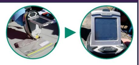
Operator places XRF equipment directly on soil sample.
