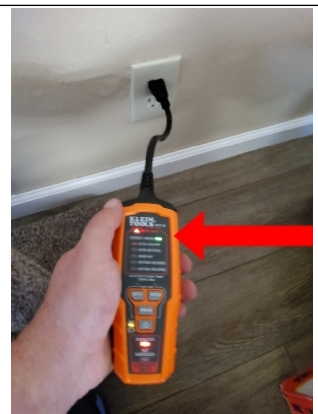
Electrical outlet shows proper grounding and polarity.
