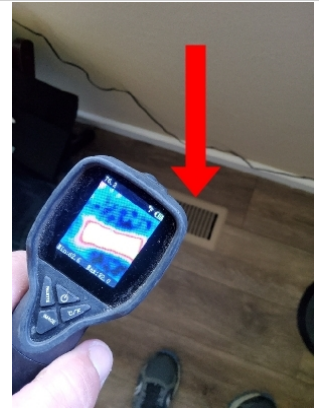
Thermal Imager shows proper HEAT distribution through floor vent.
