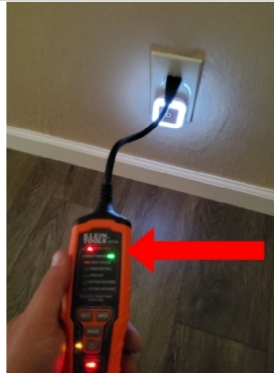
Electrical outlet shows proper grounding and polarity.
