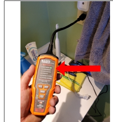
Electrical outlet shows proper grounding and polarity
