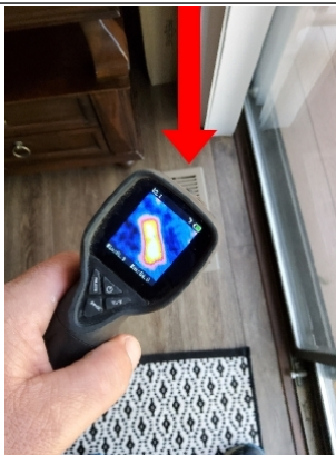
Thermal Imager shows proper HEAT distribution through floor vent.
