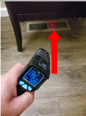
Thermal Gun shows proper AC distribution through floor vent.
