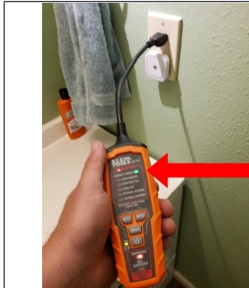
Electrical outlet shows proper grounding and polarity.
