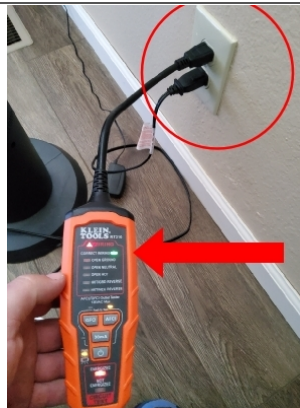
Electrical outlet shows proper grounding and polarity.
