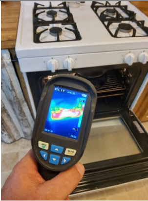
Thermal Imager shows oven properly operates.
