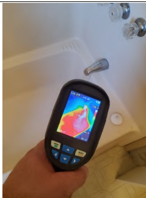
Thermal Imager shows hot water is present through spout.
