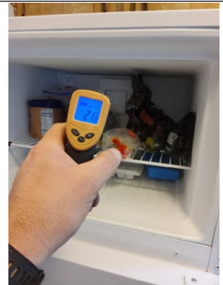
Thermal Reader shows freezer properly operates. (21 Degrees F)
