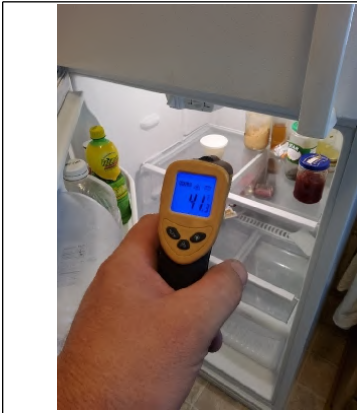
Thermal Reader shows refrigerator properly operates. (41.3 Degrees F)
