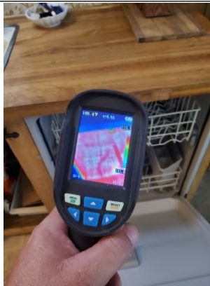
Thermal Imager shows dishwasher properly operates.
