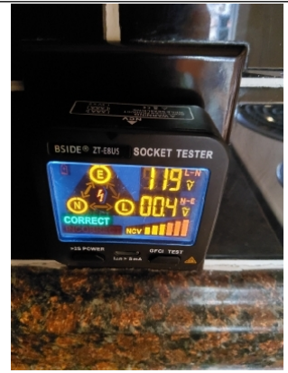
Electrical outlet shows proper grounding and polarity.
