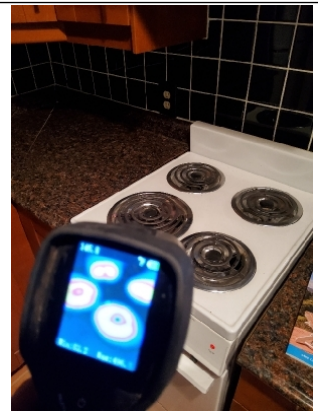
Thermal Imager shows burners properly work.
