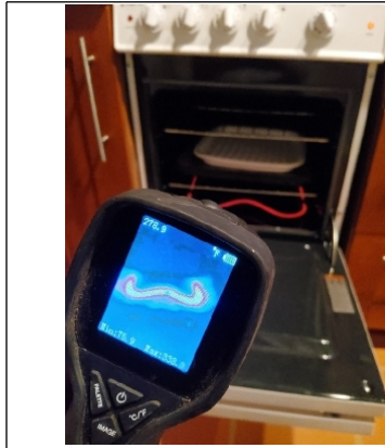
Thermal Imager shows oven properly works
