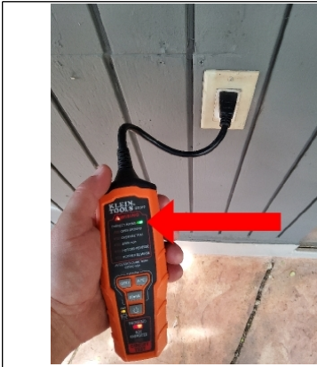
Electrical outlet shows proper grounding and polarity.
