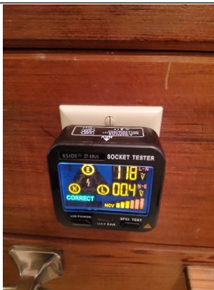
GFCI Electrical outlet shows proper grounding and polarity.
