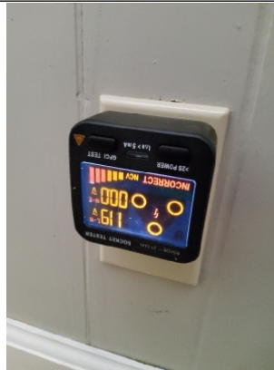
Open ground electrical outlet
