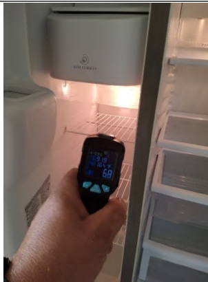
Thermal Reader shows refrigerator properly operates. (6.8 Degrees F).
