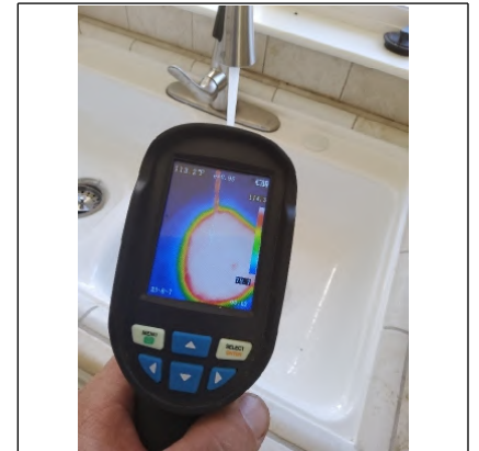
Thermal Imager shows hot water is present through faucet.
