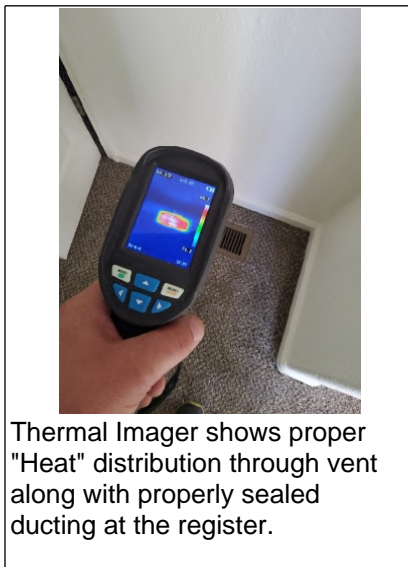
Thermal Imager shows proper "Heat" distribution through vent along with properly sealed ducting at the register.
