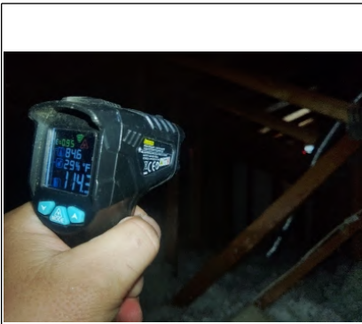
Thermal Reader shows 125.4 Degrees F at the eave vent location this shows there is proper ventilation and a moderate heat index.
