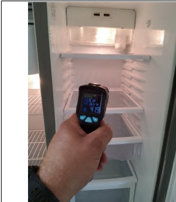
Thermal Reader shows refrigerator properly operates. (41.9 Degrees F).
