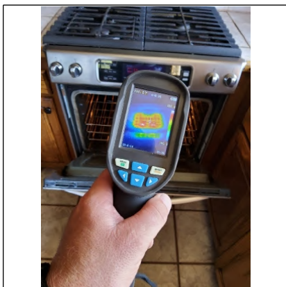
Thermal Imager shows oven properly operates.
