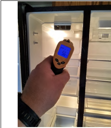
Thermal Reader shows 56.1 degrees F on freezer. This is most likely just on a high setting as its not being used.
