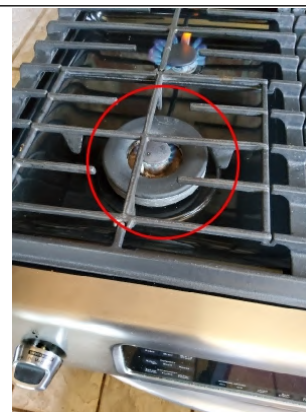
Noted burner has a low flame. Recommend having repaired by an Appliance Specialist.
