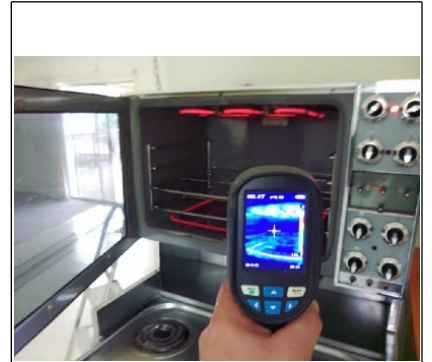
Thermal Imager shows oven properly operates.
