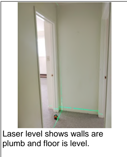
Laser level shows walls are plumb and floor is level.
