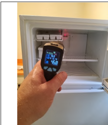
Refrigerator was only plugged in for 30 minutes but does show proper operation. (46.8 Degrees F in freezer)
