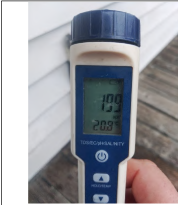
Water level shows 199 PPM which is considered to be hard water.
