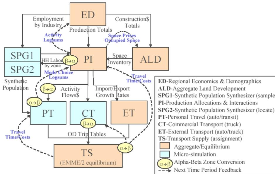
FIGURE 27 Sequence of modules in transitional models.
