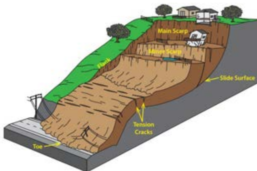
Figure 130: Diagram of an Idealized Landslide with Commonly Used Terminology 152
